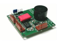
EZ-TILT-2000 rev-2 advanced programmable dual/single axis LINEAR Analog/Digital output tilt module is built around a customized state of the art CMOS Microprocessor. A 2"x 2" assembled PCB provides concurrent Analog, PWM and RS-232 inclination information in two axis of tilt.
